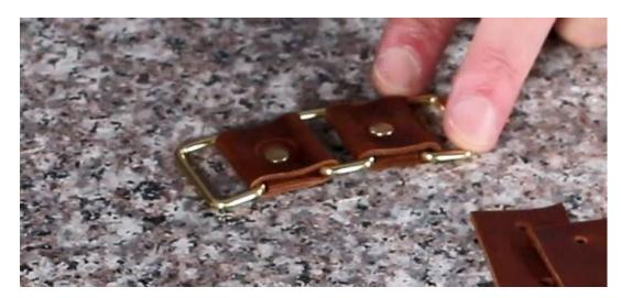
7. When enough segments have been completed, take 2 additional pieces 1" x 2 ½". These will be our "tabs" for Snaps. Punch one end hole and the center hole just like the segment pieces. Punch a hole on the other end at ¾" in from the end (You can use your Awl to mark ¾" before you punch it); then, punch a Round Strap End Punch on this end only for both pieces.
