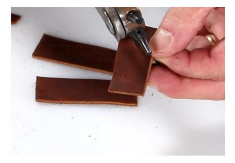
3. Punch an additional hole  $\frac{1}{2}$ " in from each end. This should give us three holes.
