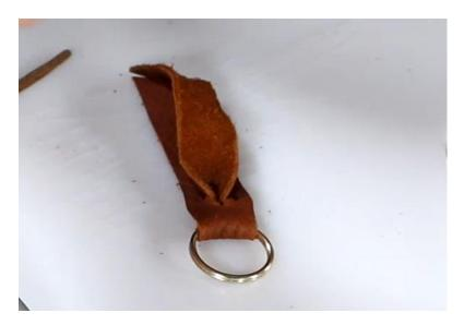
5. Cut a slit lengthwise on the front strap roughly %" below the last cut and roughly %" long.
