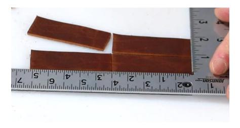
2. Take one of these pieces and fold in half, and this will give us the center of the strap. Using your Economy Punch, punch a hole on this line centered widthwise.
