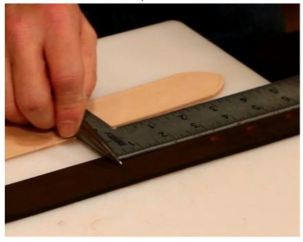
19. Place the tip of your English Point Strap End Punch on the vertical line mark. The tip should face away from your size holes. To punch your belt tip, hit the end of your English Point Strap End Punch with your Polyhead Mallet.
