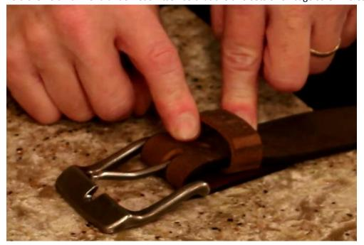
5. While holding the bend back in place, flip your Belt Blank over and let the Buckle hang off the edge of your Tooling Slab or workbench.
