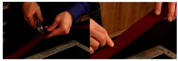
13. It's now to time to begin preparing the belt for the 4 Conchos. Lay your Measuring Tape vertically above your belt, with 0" starting at the Chicago Screw furthest away from the buckle. Measure the length from this point to your first size hole.
