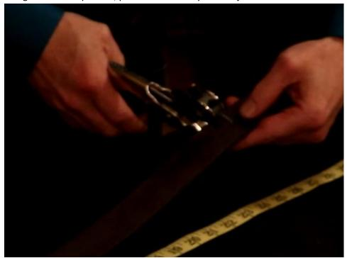
17. Screw the Conchos in the 4 holes you have just made. \*Tip: To ensure the Conchos don't work themselves out of the belt over time, add a little glue to the female end before twisting in the male end of the concho.
