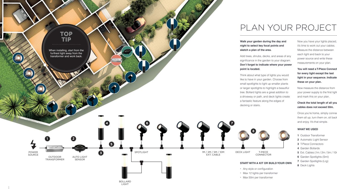
Now you have your lights placed, it's time to work out your cables. Measure the distance between each light and back to your power source and write these measurements on your plan.
