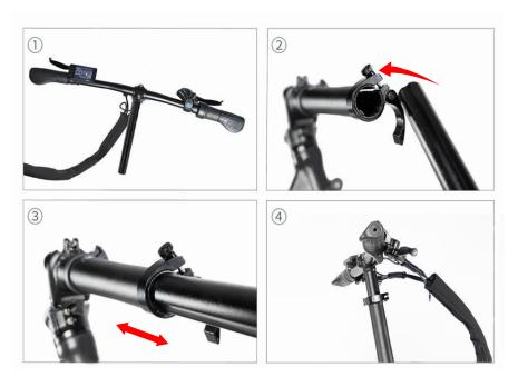
**Step 1:** Insert the stem of the handlebar into the top tube along the groove.
