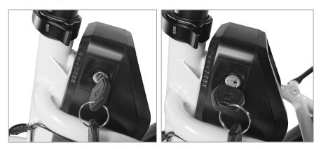
**Step 1:** Turn the key to lock/unlock the battery on bike according to the position attached to the battery as the picture shown.
