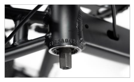
There is a serial number attached on head-tube or on the bottom axis connecting the pedals as shown in the following picture. Please take a picture ahead once you received the bike. You may be asked for a picture of your bike's serial number as a part of warranty requests and may also be asked to provide this number to law enforcement provided that your bike is stolen.
