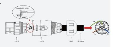
3. Plug the AC port Part 2 into Part 1 once the wiring is complete, then screw on Part 3 to complete the AC extension cable.
