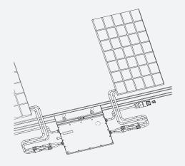
Fig.1 Microinverter installation position
