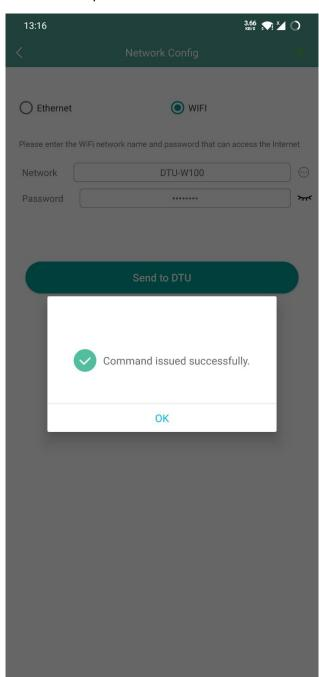
Step4: Back to your phone setting page, turn off the WiFi option and replug the DTU power. Wait for 40 seconds,
