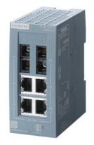
SCALANCE XB004-2LD unmanaged Industrial Ethernet Switch for 10/100 Mbit/s; for setting up small star and line topologies; LED diagnostics, IP20, 24 V AC/DC power supply, with 4x 10/100 Mbit/s twisted pair ports with RJ45 sockets; 2 x 100 Mbit/s single-mode glass fiber-optic cable port with SC socket; manual available as a download .
