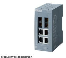
SCALANCE XB004-2 unmanaged Industrial Ethernet Switch for 10/100 Mbit/s; for setting up small star and line topologies; LED diagnostics, IP20, 24 V DC power supply, with 4x 10/100 Mbit/s twisted pair ports with RJ45 sockets; 2x 100 Mbit/s multimode glass fiber-optic cable port with SC socket; manual available as a download.
