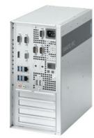
SIMATIC IPC527G (Box PC); Core i5-6500 (4C/4T, 3.2 (3.6) GHz); 256 GB SSD, internal; 8 GB DDR4; Windows 10 Enterprise 2016 LTSB 2x Gigabit Ethernet (IE/PN); 1x display port, 1x VGA; 4x USB 3.0, 2x USB 2.0; 2x RS232/485/422 (can be selected); 2x RS232, 1x 8bit DIO, 2x PCI; 1x PCIe x16, 1x PCIe x1; 100/240 V AC power supply without line cable
