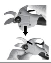
1.Use an Allen wrench to rotate the screw counterclockwise and loosen it, then remove the casing.
