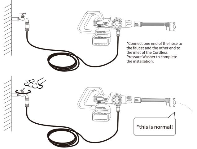
After connecting to the faucet, you need to turn on the faucet switch to use it normally. When you turn on the faucet switch, a small amount of water will come out of the pressure washer nozzle (this is normal!). It means that the pressure washer hose and the machine are already filled with water, and you can proceed with normal operation at this point.
