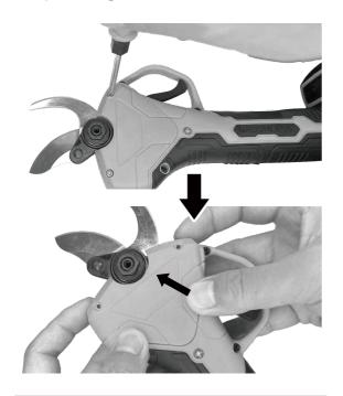
1. Unscrew the screws with a Phillips screwdriver and push the blade gear guard upwards to remove the gear guard.
