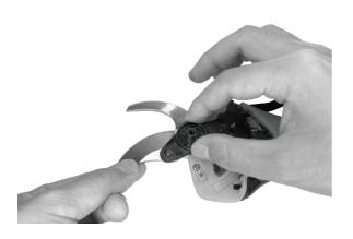
3. Remove the upper blade (if the blade is too tight, tap it with an Allen socket wrench to loosen it and remove it).
