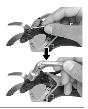
2. Unscrew the fixed shaft screw counterclockwise with a suitable hexagonal wrench and remove the washer, then unscrew the shaft screw counterclockwise with a hexagonal socket wrench and remove the spacer from the shaft.
