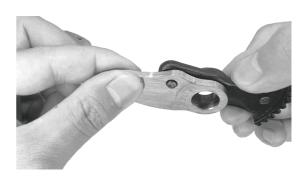
4. Separate the support arm from the upper blade (if the blade is too tight against the support arm, use an Allen socket wrench to gently tap the support arm to loosen the upper blade).
