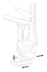
To remove the battery pack from the tool, press the release button and firmly pull the battery pack out of the tool handle.
