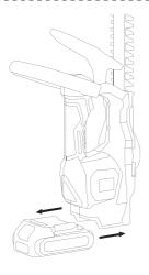
To install the battery pack into the tool handle, align the battery pack with the rails inside the tool's handle and slide it into the handle until the battery pack is firmly seated in the tool and ensure that it does not disengage.
