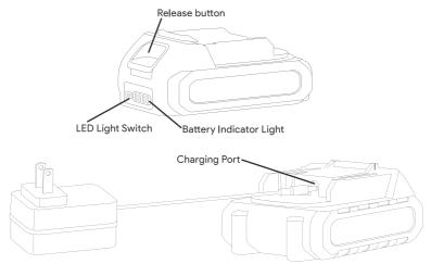
Use our included adapter to charge the battery, and it takes about 2 hours for a single full charge (note: the charging interface is at the position shown in the above figure).
