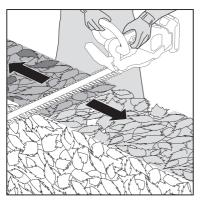
(3) Horizontal left and right cutting. (4) Up and down cutting.
