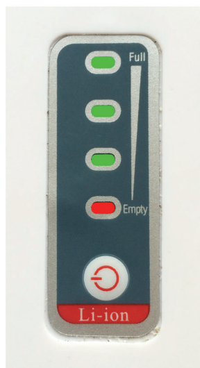
Fig 2 Battery status indicator
