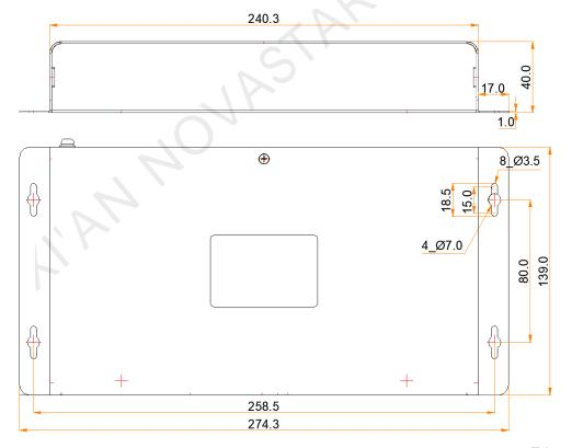
Tolerance: ±0.3 Unit: mm
