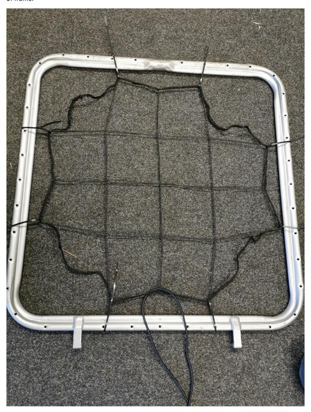
Step four – Weave the bungee in and out of the net squares and attach to the frame using the clips provided (see images for the top, corners and bottom frame when complete)
