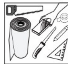
Padsaw or a fine toothed handsaw, spacer blocks, pencil, set square, 0.2mm PE film and adhesive tape.
