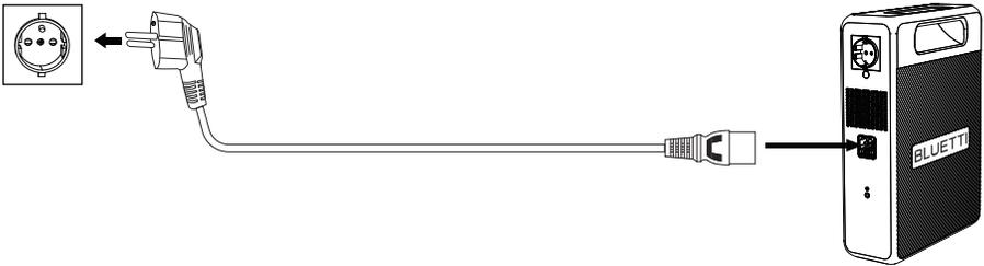
**Note:** Do not plug the unit's AC charging cable into its own AC outlets. Doing so could damage the connected device.
