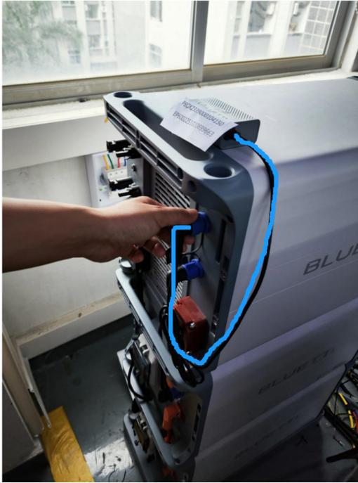
Step 3 : Remove the signal cable (connecting EP600 and B500) from the Master, i.e. the EP600 on the right.
