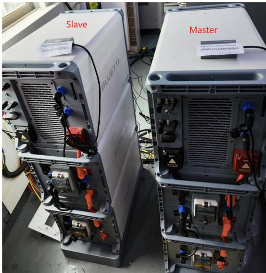
Step 2 : Remove the IOT box of the slave, i.e. the EP600 on the left.
