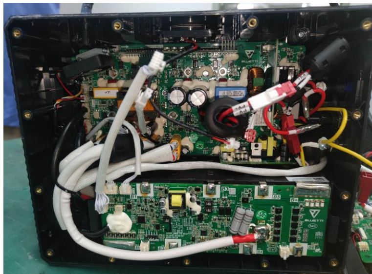
Internal view after IP6X test (there is no dust inside)
