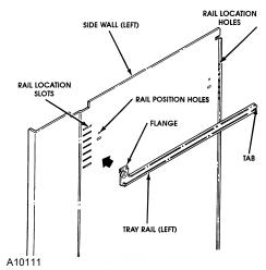
Figure 12. Removing a Tray Rail
