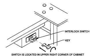
Figure 4. Location of Interlock Switch
