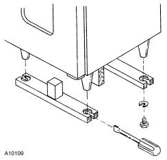
Figure 1. Removing the Knock-A-Way Supports
