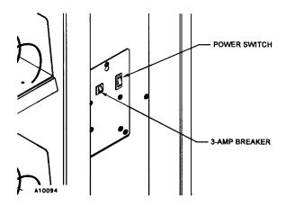
Figure 5. Power Switch and 3-Amp Breaker
