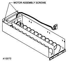
Figure 10. 2-WideTray, Motor Mount Assembly
