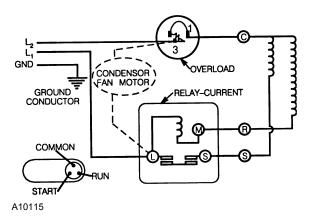
Figure 14. Compressor Schematic
