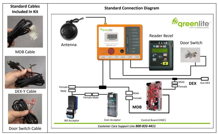
Figure 1: Illustrated Wiring Diagram
