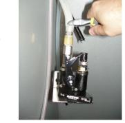
3) Select either of the 2 x #10-24 or #10-32 x 1" screws in the kit and introduce to the same threaded inserts that the original screws were removed from, screw-in a few turns only using fingers
