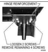
Figure 4d. Remove Left Reinforcement Plate
