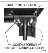
Figure 4d. Remove Left Reinforcement Plate
