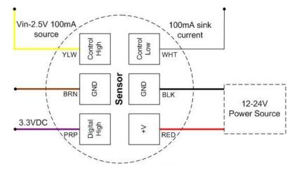
Note: If using a power pack other than PSC-AC-PP-200, connect either Control Hi or Control Low, depending on power pack relay circuitry.
