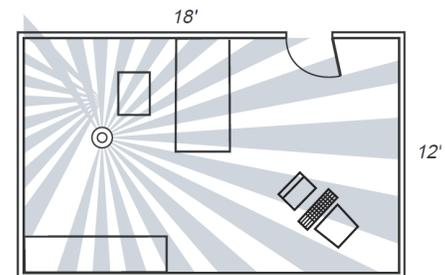
Figure 3: Open Office Dual Tech Sensor
