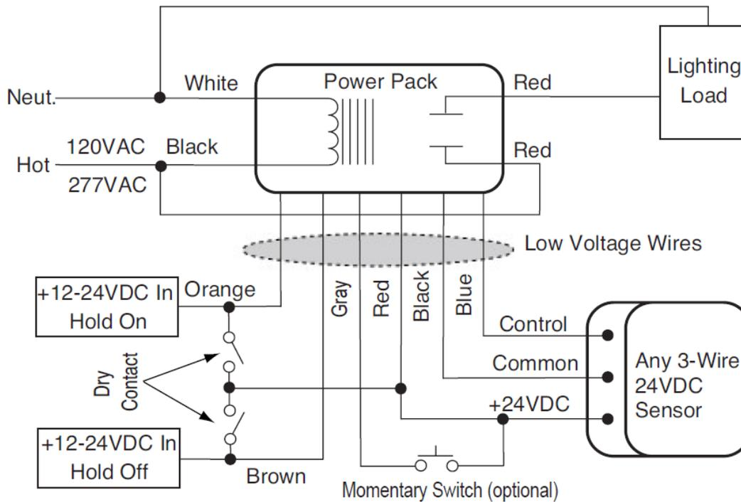
**Manual Switch Wiring & Operation**
