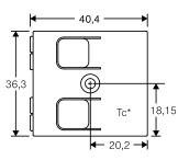
Wire info: Solid and stranded: 16-20 AWG/ 0,5-1,5 mm<sup>2</sup> Strip length: .25"/6-8 mm
