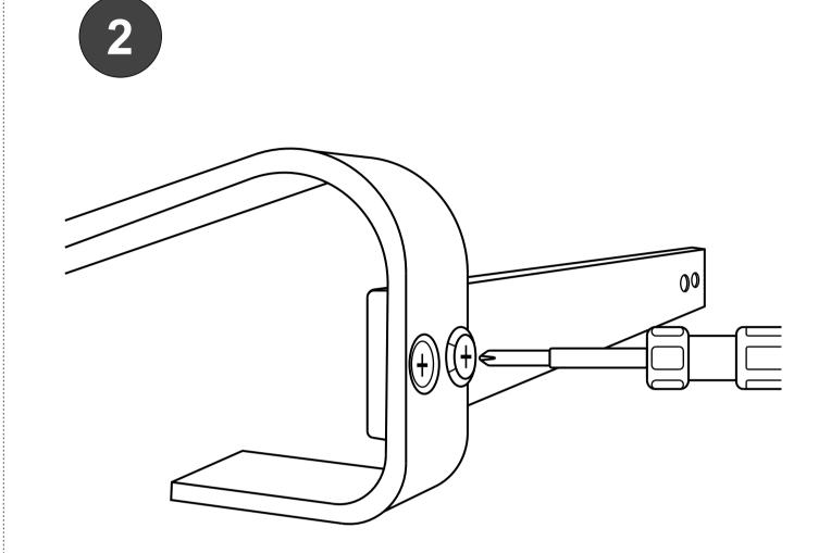
Connect the two parts shown in the picture with a screwdriver and screws.
