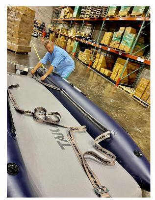
2) Run the tow straps around the lower transom bar and loop back through the buckle.
