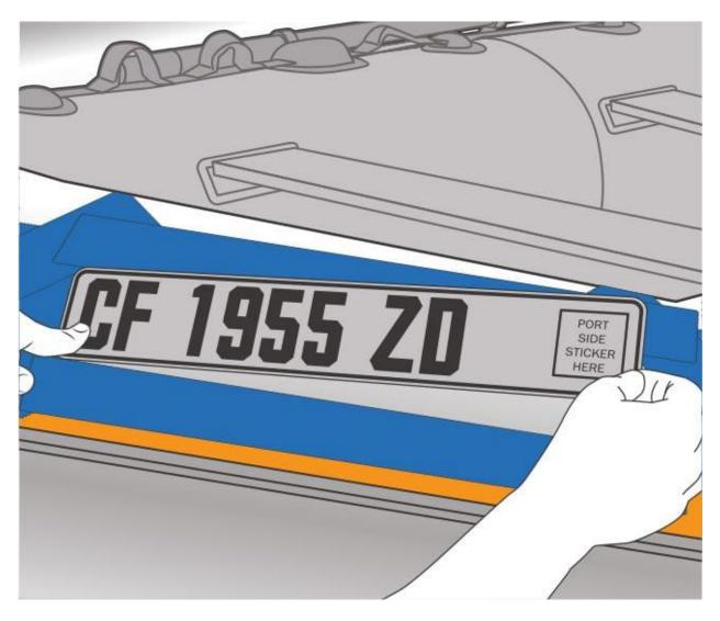
**Installing Registration Numbers on an Inflatable Boat**
