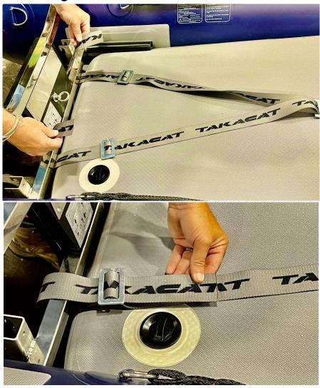
Step 4) After adjusting the length, lock the buckles by looping strap back through the buckle and connect the ring to your davit lifting system
