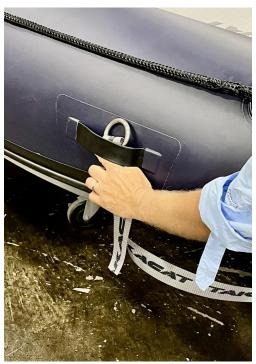
Step 2) Use the buckles to adjust strap length as needed and connect both looped rings to your davit
