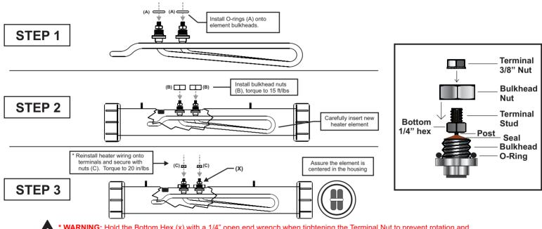
\* WARNING: Hold the Bottom Hex (x) with a 1/4" open end wrench when tightening the Terminal Nut to prevent rotation and damage to the epoxy end seal.
