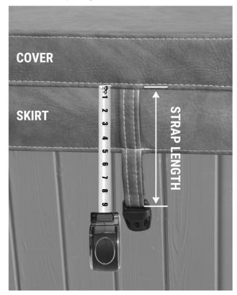
The strap length is measured from the bottom of the cover (which is the top of the spa's rim) to the top of the latch, as illustrated. In our example, the straps are 9" long, extending 4" below the skirt.
