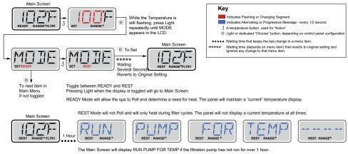
The Main Screen will display normally during Filter Cycles or when the spa is in use
