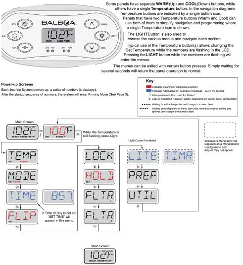
Waiting Several Seconds in the Main Menu will allow the display to revert to the Main Screen. Most changes are not saved unless Light is pressed. Refer to Key above.
