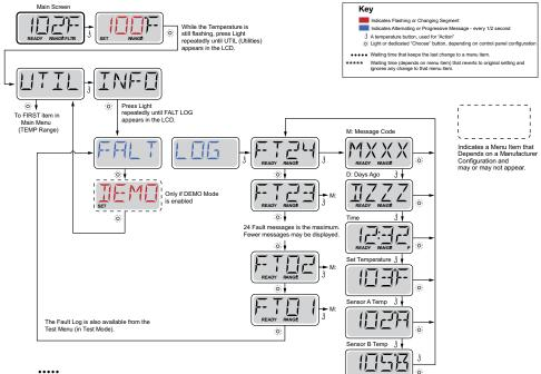
••••• Waiting several seconds inside the Fault Log Menu will allow the screen to return to normal operation.
