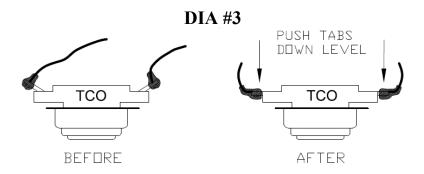
Step #6 Assemble box and reconnect TCO control wires. Failure to connect the TCO wiring will cause a system error and stop heater operation.
