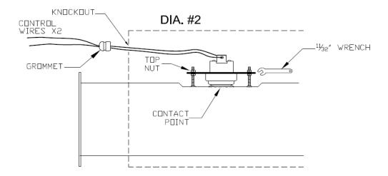
Step #3 Install top nuts and run down until TCO mounting plate is tightly captured between both top and bottom nuts as shown in diagram #2
