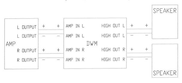
Parallel connection for full-range floor-standing models, with DWM bass augmentation (Use only high current amplifiers).
