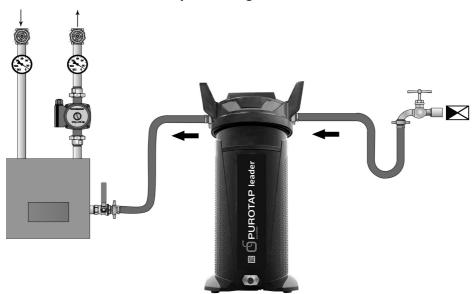
This connection version is suitable for filling heating systems with demineralised water.
