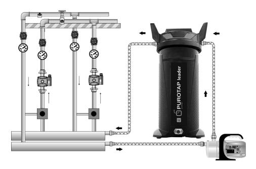
This process is also suitable for subsequently demineralising systems with an excessively high salt content according to boiler manufacturer specifications or guidelines.
