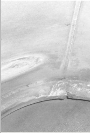
Over heating, stress crack
