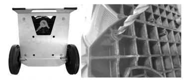
Drill out the 4 holes to ø7 mm.
