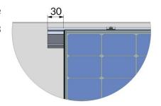
Install 4 MOUNTING CLAMPS (E) for the panel to anchor it to the structure. Install 2 Clamps on the upper panel rail and 2 Clamps on the lower panel rail. They will be positioned 200 mm from the end of the panel as shown in the figure.
