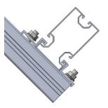
• IMPORTANT: The lower clamp must be positioned EXACTLY on the edge of the vertical profile (A), as shown in the figure.
