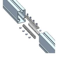
• Place the LOWER PANEL RAIL (B) on the VERTICAL PROFILES (A) and anchor it using two pre-assembled mounting clamps, as shown in the figure.
