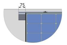
• Install 4 MOUNTING CLAMPS (E) for each panel to anchor them to the structure. Install 2 Clamps on the upper panel rail and 2 Clamps on the lower panel rail. They will be positioned 200 mm from the end of each panel as shown in the figure.
