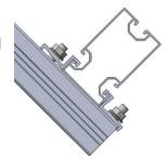
• IMPORTANT: The lower clamp must be positioned EXACTLY on the edge of the vertical profile (A), as shown in the figure.
