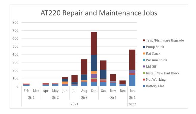
The first major challenges started arising with the traps around 3 months after they were activated in the field. Following a project wide firmware upgrade and repairs, the issues we have experienced to date have largely been resolved satisfactorily. We continue to work with NZ AutoTraps on the pump/lure issue and resolving other issues as they arise.
