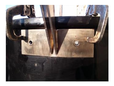
Step 2: Using your locking pliers secure the hinge to the middle section. Make sure the hinge is level and parallel to the lip of the middle section.
