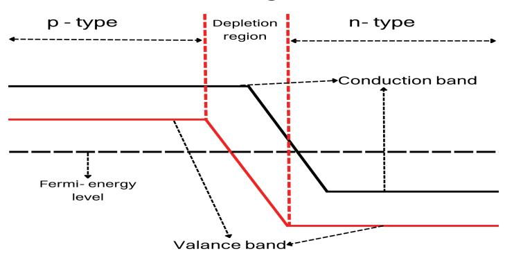
Figure 1: Energy band structure of a PN junction.
