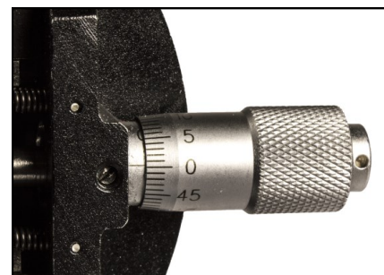
Moving jaw range is 0-2.50 mm
