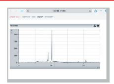
When using the HD additive X-ray (554 835), the Bragg spectrum already shows fine splitting of the KB line in the first order and fine splitting of the Ka line in the second order if a LiF crystal is used instead of the NaCl crystal.
