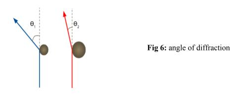
The angle of diffraction for small particles ( $\theta_1$ ) is bigger than the diffraction angle of bigger particles ( $\theta_2$ ).
