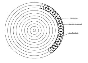
Fig 3: wavefronts can be regarded to be composed of a collection of closely spaced, coherent point sources
