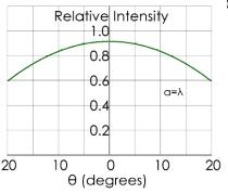
) bstacle equal to the wavelength of the light.  $a=\lambda$
