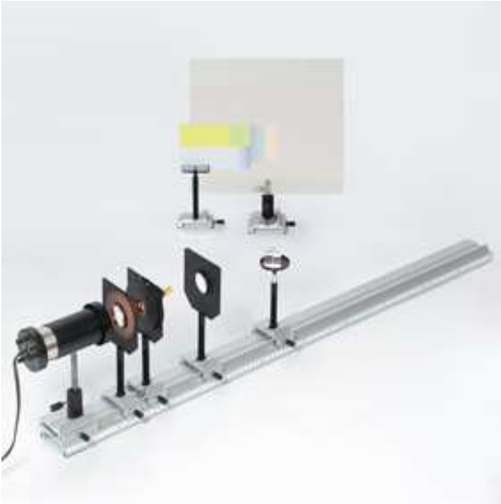
Detection of ultraviolet radiation in the continuous spectrum of an incandescent lamp.
