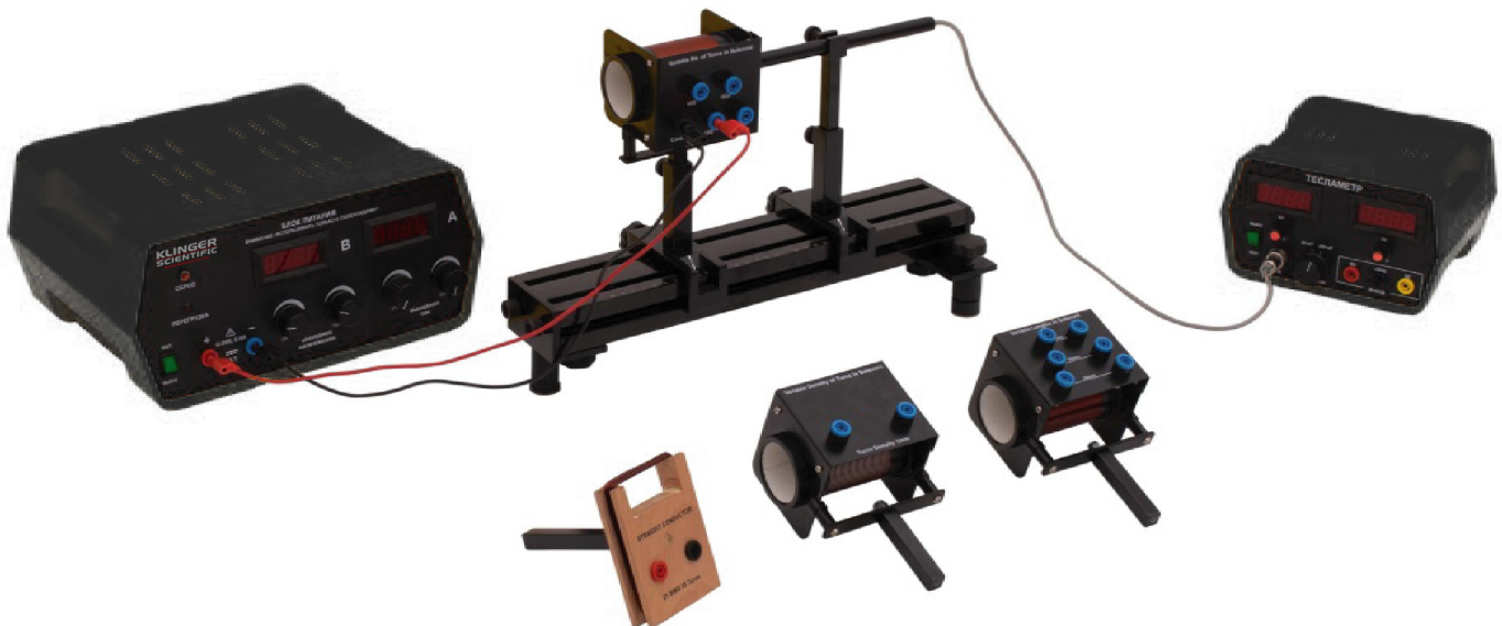
Image 5. Experimental installation with conductors of various configurations and axial Hall sensor
